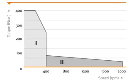
A two-gear stage design enables different torque ranges for flexible applications with high and low viscous media
