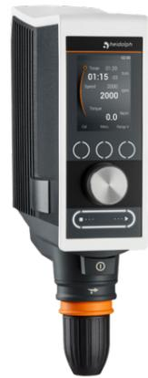
USB and RS 232 interfaces allow for documentation and reproducibility, e.g. with the free Hei-Control software (for up to four devices)
