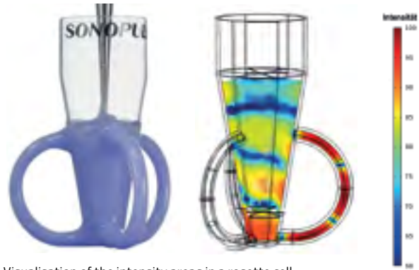
Visualisation of the intensity areas in a rosette cell Source reference: Beuth Hochschule Berlin
