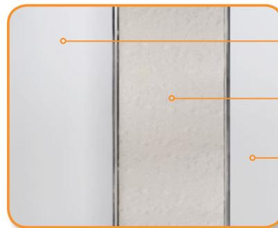
5" thick polyurethane foam is placed in the main cabinet and 4.5" on the door.
