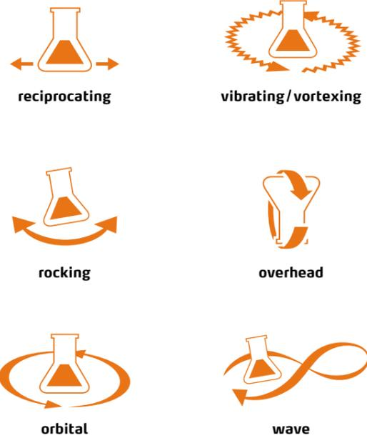
Six different shaking movements – from one- to three-dimensional. Individual motions additionally vary in their movement amplitudes and tilt angles.
