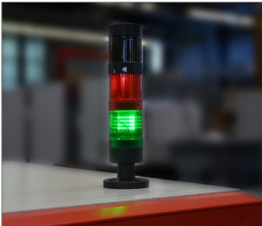
Program sequence display using indicator lamps
