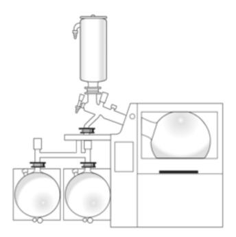
Hei-VAP Industrial model with glassware KC - Condensate trap for low-boiling solvents; cooling by dry-ice
