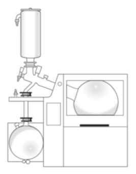
Hei-VAP Industrial B model with glassware K - Condensate trap for low-boiling solvents; cooling by dry-ice
