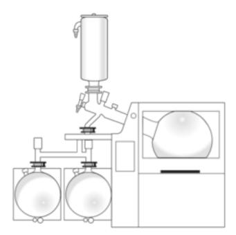
Hei-VAP Industrial B model with glassware KC - Condensate trap for low-boiling solvents; cooling by dry-ice
