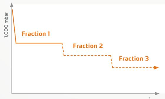
The DAA allows you to start a fully automated distillation process already during the heat-up phase of the heating bath. The system vacuum is dynamically adjusted to the changing heating bath temperatures until the heating bath has reached its defined temperature.
