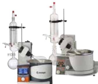
**Ground-free condenser:** Ventilation cap with PTFE inlay and threaded connection prevents stuck glass
