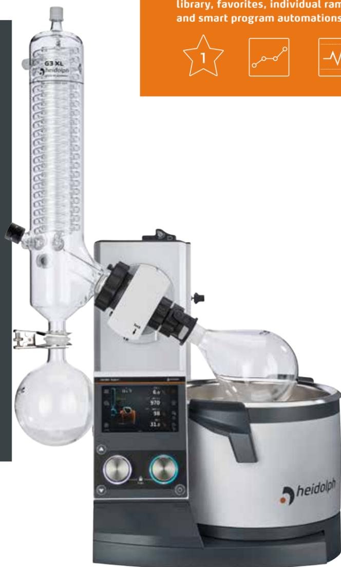
Central control panel for direct regulation of any vacuum source – in conjunction with a Hei-CHILL recirculation chiller also the cooling temperature. With solvent library, favorites, individual ramps and smart program automations.
