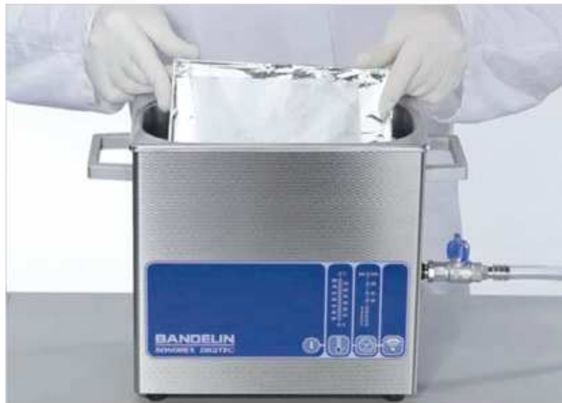
Foil stretched on a foil test frame
