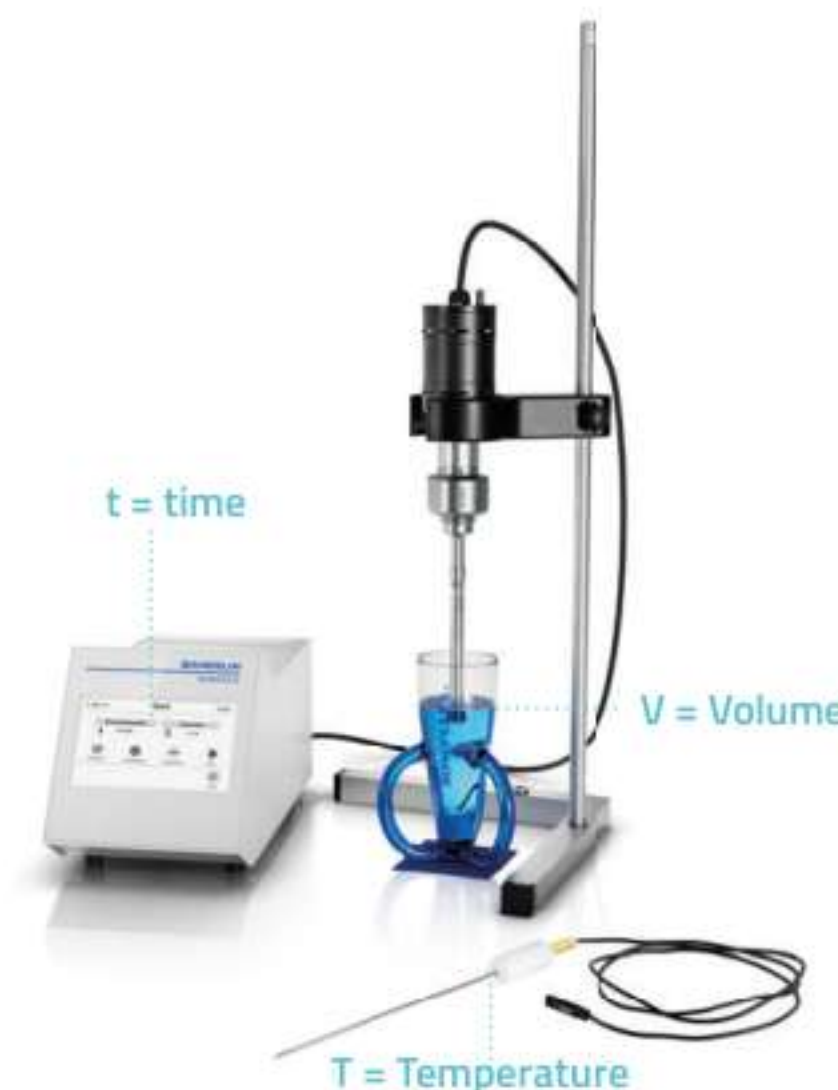
Illustration of the experimental set-up of a calorimetric measurement to determine performance
