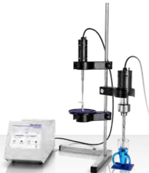
Sonication of two samples on one stand
