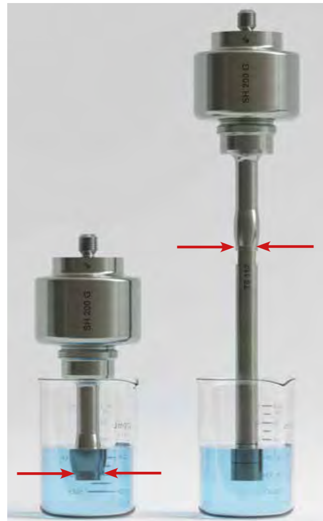
Screw connection horn/titanium disc and horn/probe, cylindrical
