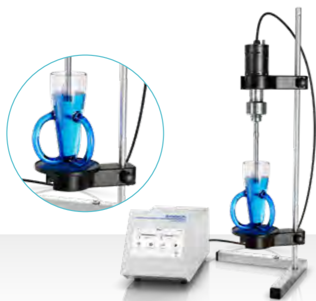
Direct sonication with supporting table
