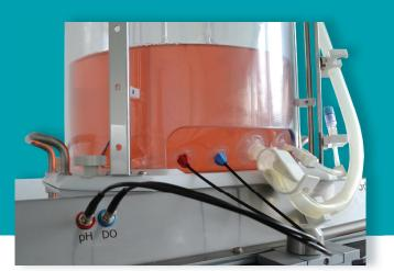
The SB10-X is an orbital shaken benchtop bioreactor system for the cultivation of human, mammalian and plant cells in a single-use bag. It consists of six modules (excluding the bag) and has a working volume from 4 litres up to 12 litres. The SB10-X can be used in research, process development or as a pilot scale bioreactor.
