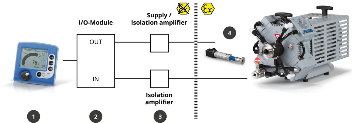
**1 CVC 3000** Installation outside of the EX-area, without integrated sensor
