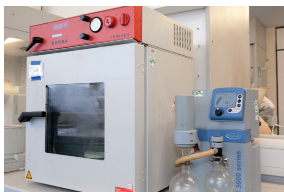
Drying cabinet with pumping unit
