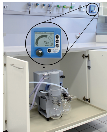
Vacuum network pumping unit under the exhaust hood, with solvent recovery, operation via the media console
