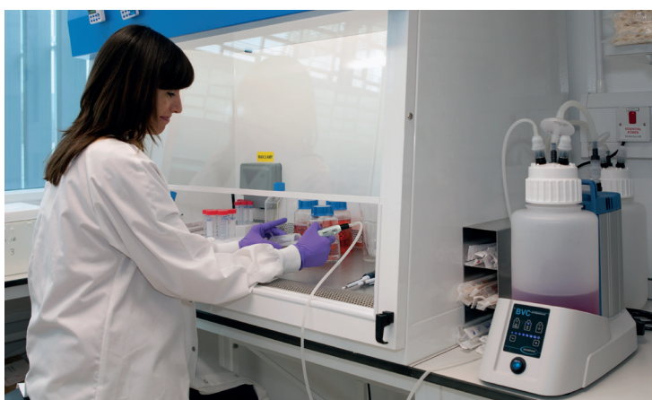
Stand-alone solution: Rough vacuum, aspiration of liquids
