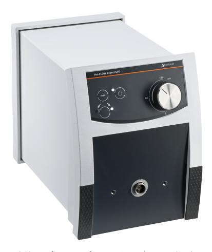
This model has a flow rate of 2.0-4,056 ml/min and is designed for operation with single-channel pump heads. The analog interface makes it possible that all functions can be controlled externally. A control accuracy of  $\pm 0.5\%$  and a conveyor speed of 24 to 600 rpm provide optimum process conditions. In addition, sensitive media can be protected from influence by using the optional foot switch.
