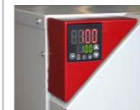
Controller with 7-segment display
