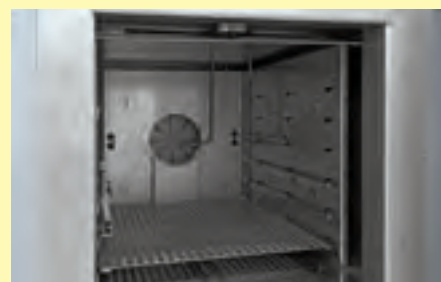
Interior with metal shelf, thermocouples and pressure monitoring
