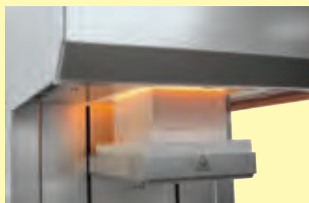
Electrically driven lift-bottom
