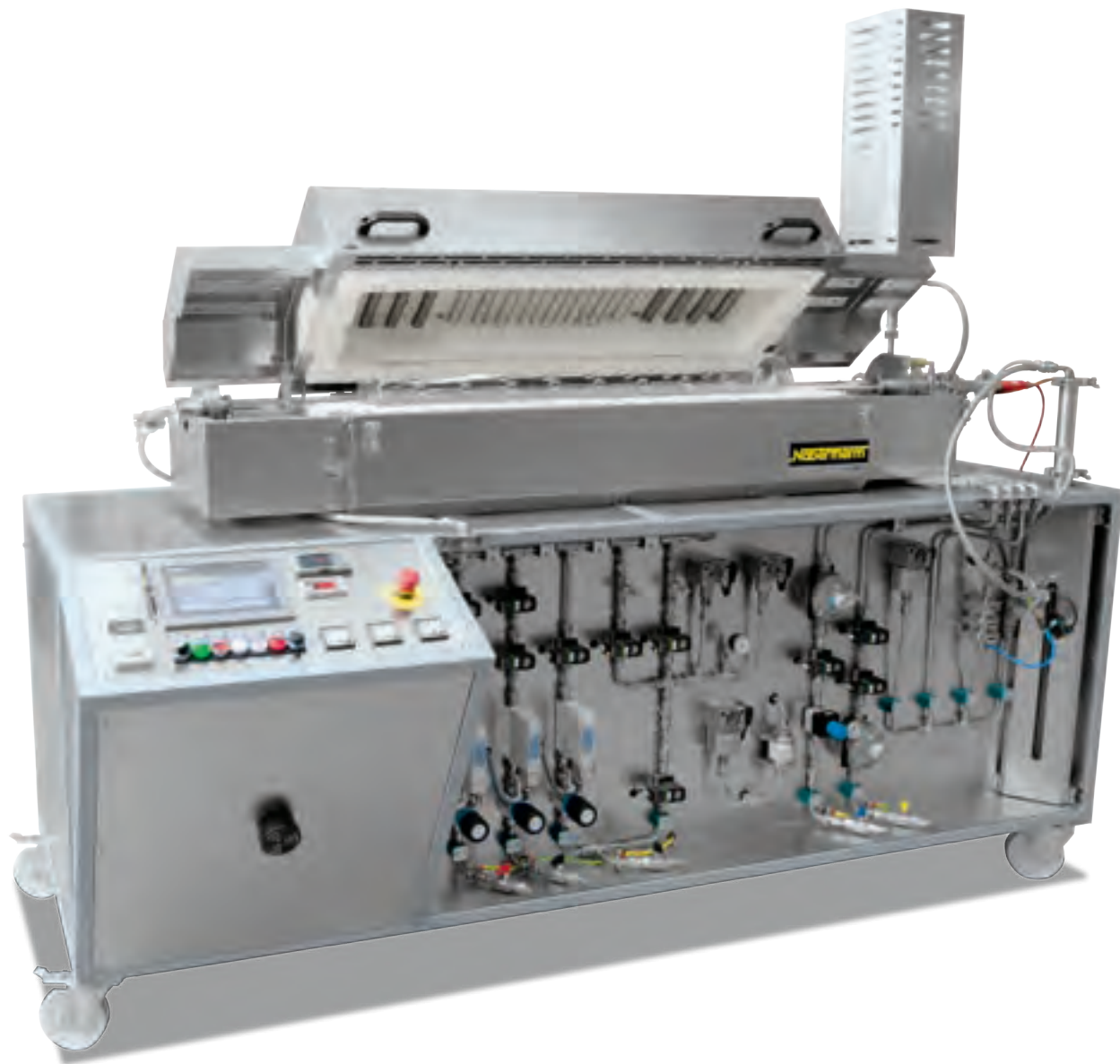
RSRB 170/1000/11 H 2 with gas supply package 4 for hydrogen application
