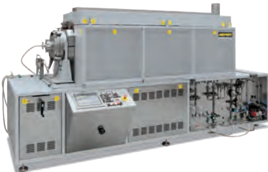
RS 320/2000/09 H 2 with three-zone control for heat treatment of precious metals
