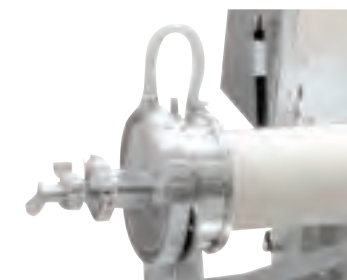
Water-cooled vacuum flange (gas supply system 2)
