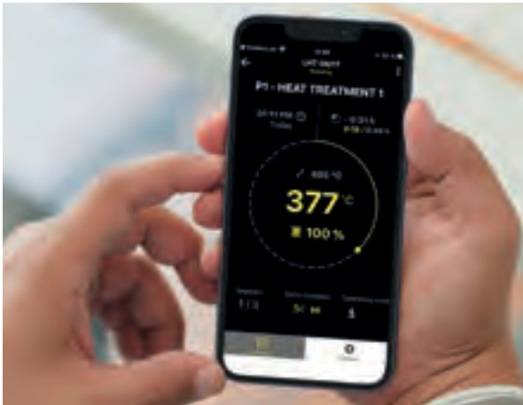
Display of program progress for each furnace
