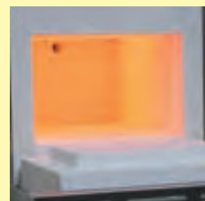
Muffle heated from four sides
