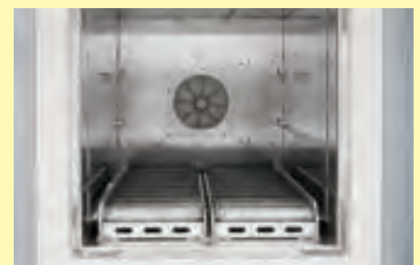
Roller conveyor in furnace chamber
