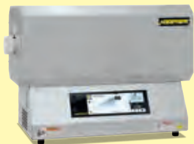
Tube furnace R 50/500/12 with three zone control
