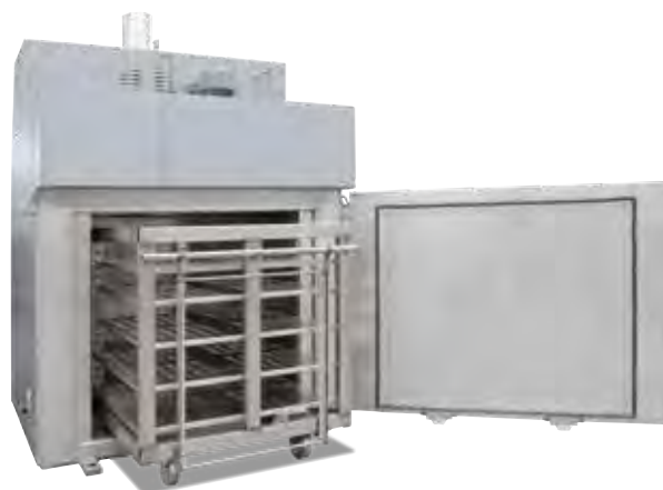
Chamber oven KTR 1500 with charging cart
