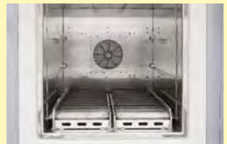
Roller conveyor in furnace chamber
