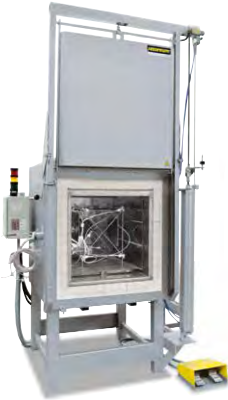
Holding frame for measurement of temperature uniformity
