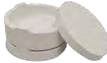
Round Saggars (Ø 115 mm) for Furnaces LHT/LB, Tmax 1650 °C
