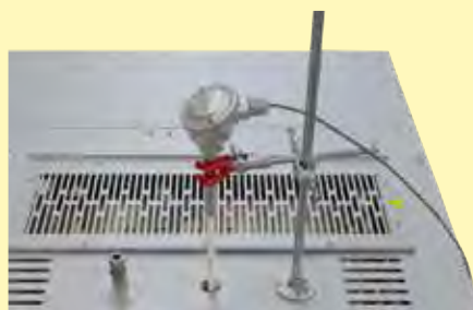
Thermocouple port in the ceiling with tripod
