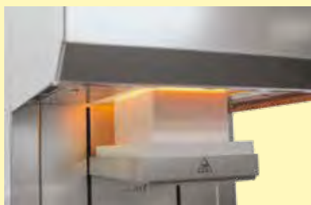
Electrically driven lift-bottom
