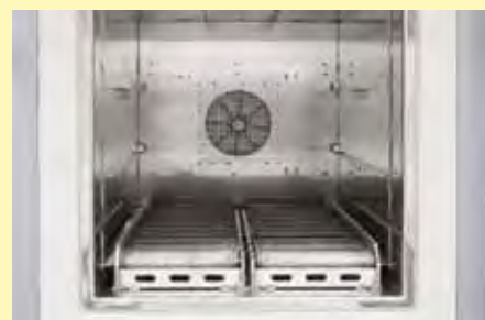
Roller conveyor in furnace chamber
