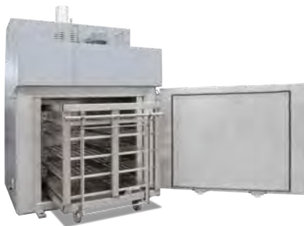
Chamber oven KTR 1500 with charging cart
