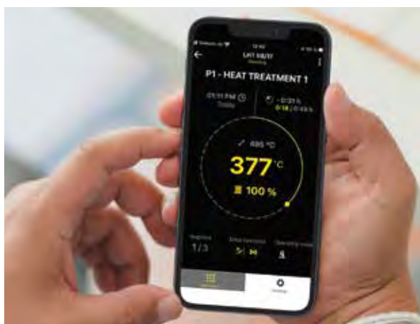
Display of program progress for each furnace
