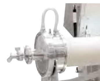
Water-cooled vacuum flange (gas supply system 2)
