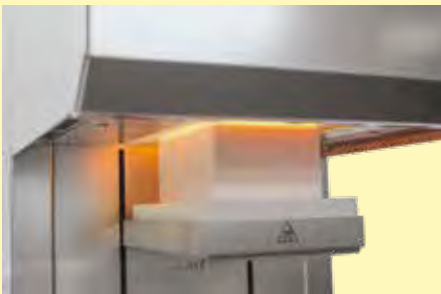
Electrically driven lift-bottom
