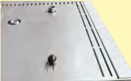
Adjustable exhaust port in the furnace ceiling
